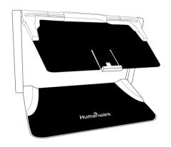
3. Hold your tablet with the screen facing you, ensuring the HumanWare logo is at the top. Carefully insert the tablet into the slot and slide it forward until you reach the back end of the slot. Push the bottom part of the tablet down; you will hear a *click* indicating that your tablet is locked into place.
