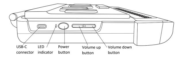
Connect your recharge cable's USB connector into the power adaptor, then plug the power adaptor into a power outlet. The connector and cable are included with your BrailleNote Touch. Use the provided power adaptor for optimal recharge.
