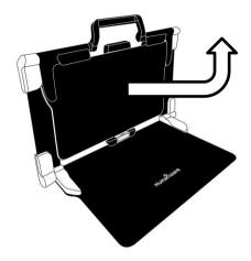
3. Hold your tablet with the screen side facing you, making sure the HumanWare logo is at the top. Carefully insert the top of your tablet into the slot and slide it forward until you reach the back end of the slot. Push the bottom part of the tablet down; you will hear a click indicating that your tablet is fastened.
