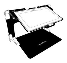
4. Connect the power supply cable to the recharge port and plug it to an outlet. The recharge port is located on the right side of the tablet. Allow the tablet to recharge until the battery is full.
