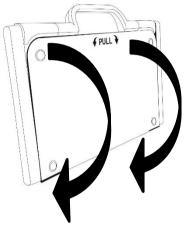
**2.** Next, unfold the top panel until it is roughly parallel with the lower panel.
