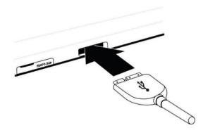
IMPORTANT: Use caution while inserting the cable into the Recharge Port.
