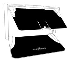
3. Hold your tablet with the screen side facing you, making sure the Samsung logo is upside down. Carefully insert your tablet into the slot and slide it forward until you reach the back end of the slot. Lock the front bracket to fasten your tablet onto the folding stand.
